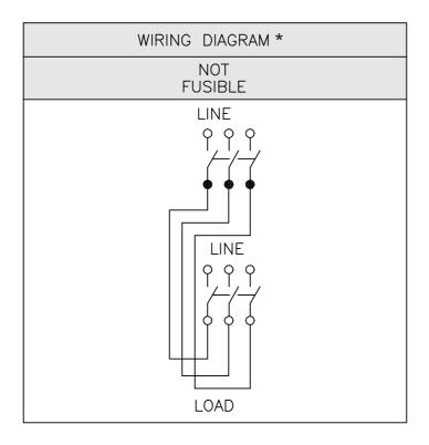
DTU321 DTU362DTU361 DTU323DTU322 DTU363
