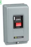
Manual Starter, integral horsepower, NEMA M0, 600 VAC, 3 pole, 5 HP at 380/575 VAC, three phase, no indicator, NEMA 1
