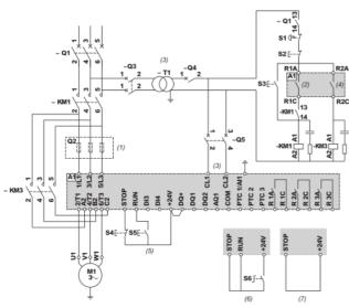
(1) : Installation of additional fast-acting fuses to upgrade to type 2 coordination according to IEC 60947-4-2.
